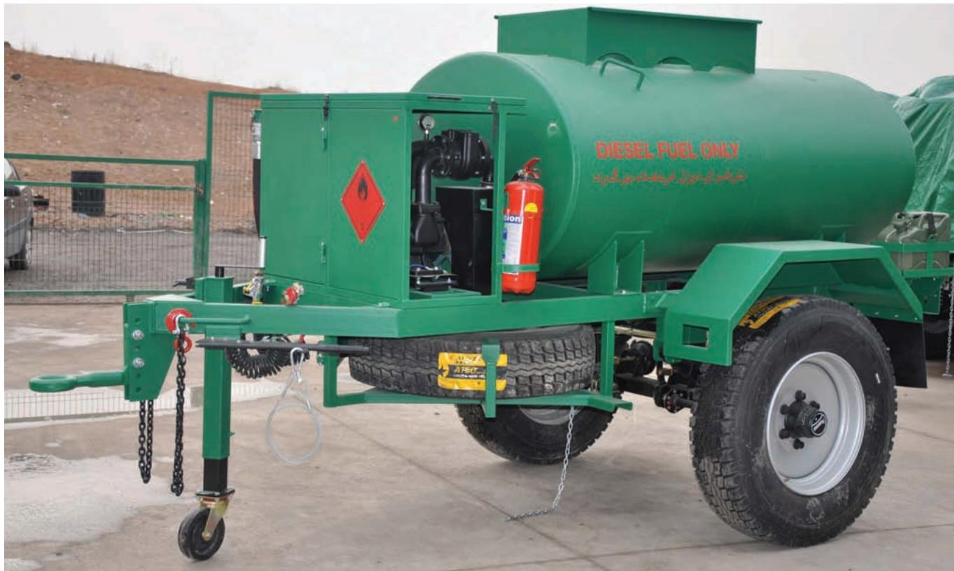
These trailers are designed for refueling vehicles and equipment on site. Their various specifications allow them to be used for either transport of fuel on/off roads or for transport and static refueling on location.
